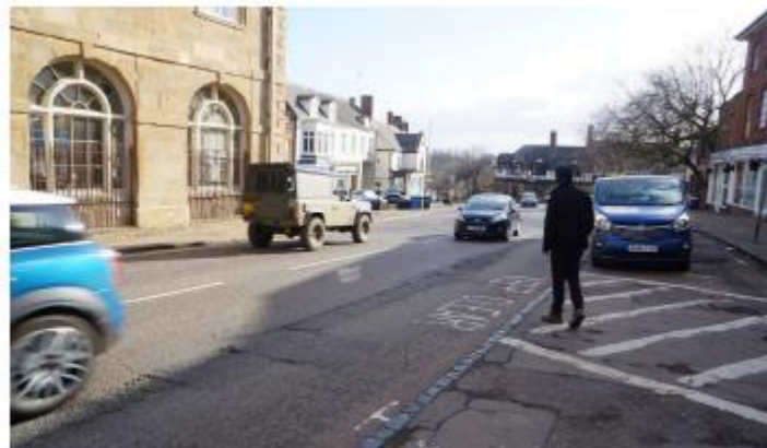
Wide carriageway incorporating parking bays makes it difficult for people to cross the road
